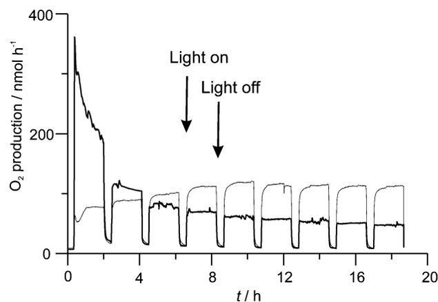
**Fig. 16** Photo electrochemical experiment, illustrating the difference of the oxidation of water to  $\text{O}_2$  for a  $\text{AgCl}$  surface modified zeolite-A electrode (bold), and for a  $\text{AgCl}$  layer on a gold modified conducting glass electrode. The corresponding current, about 8  $\mu\text{A}$  during light period for the layer on gold, 0 for the zeolite layer, is not shown; see refs. 45 and 46.
