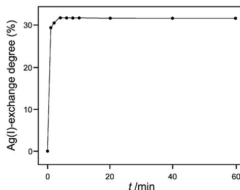
**Fig. 4**  $\text{Ag}^+$ -exchange degree of zeolite A as a function of the exchange time at 20 °C. A 9.1 mg sample of zeolite A was added to 200 mL of an aqueous 1 M  $\text{NaNO}_3$  + 1 mM  $\text{AgNO}_3$  solution. The  $\text{Ag}^+$  content of the aqueous phase was measured by means of a  $\text{Ag}^+$  ion selective electrode.<sup>30</sup>
