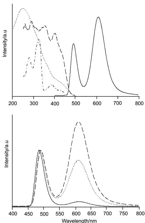
**Fig. 13** Top:  $\text{Ag}_2\text{S-CaA-1}$ : luminescence (solid) and excitation spectra (dashed observed at 620 nm, dash dot observed at 490 nm) at  $-190^\circ\text{C}$ , and diffuse reflectance spectrum (Kubelka-Munk) at room temperature. Bottom: Luminescence spectra of  $\text{Ag}_2\text{S-CaA-x}$  with  $x = 0.1$  (solid),  $x = 0.75$  (dot), and  $x = 1$  (dashed) after excitation at 320 nm. The spectra are scaled to the same height of the short wavelength band.
