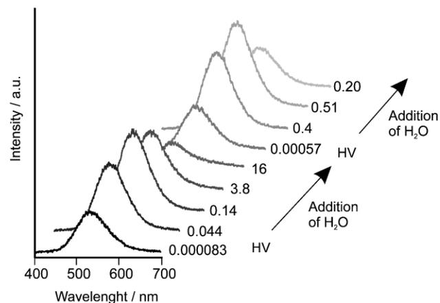
**Fig. 8** Luminescence spectra of  $Cu_{0.3}H_{9.3}Na_{67.4}X$  as a function of the degree of hydration measured at room temperature after excitation at  $355\text{ nm}$ . Two evacuation–hydration cycles are shown. The numbers on the right side of the spectra are the pressure in the sample compartment in mbar. HV means  $30\text{ min}$  of evacuation at room temperature.<sup>26</sup>
