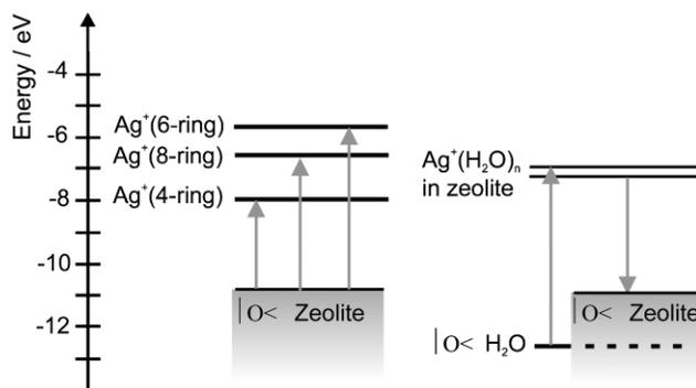
**Fig. 10** State diagram of  $\text{Ag}^{+}$ -loaded zeolite A. On the left side we show the levels observed in room temperature activated zeolites in which all three sites are occupied by silver ions, while the scheme on the right side corresponds to situations typically observed in  $\text{Ag}^{+}_x\text{Ca}^{2+}_{6-0.5x}\text{A}$  materials containing some water.
