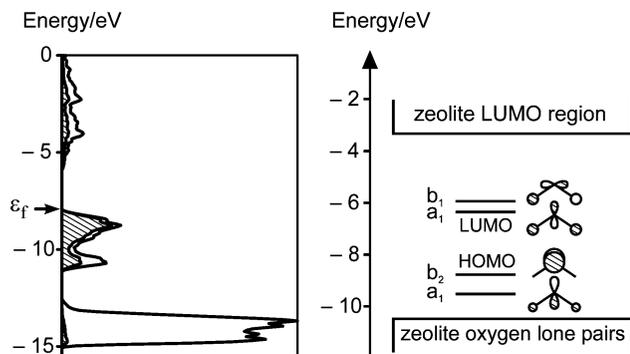
**Fig. 11** *Left*: Density of states (DOS) plot of  $\alpha\text{-Ag}_2\text{S}$ . The hatched region indicates the contribution of sulfur 3p-states. The Fermi level  $\epsilon_f$  is marked by an arrow. *Right*: HOMO-LUMO region of a  $\text{Ag}_2\text{S}$  molecule in comparison to the HOMO-LUMO region of zeolite A.
