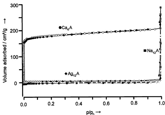
**Fig. 3** Argon adsorption isotherm of  $\text{Ca}_6\text{A}$ -,  $\text{Ag}_{12}\text{A}$ -, and  $\text{Na}_{12}\text{A}$ -zeolites, measured at the boiling point of Ar (87 K).  $p/p_0$  is the relative pressure;  $p_0$  is the saturation pressure of Ar.
