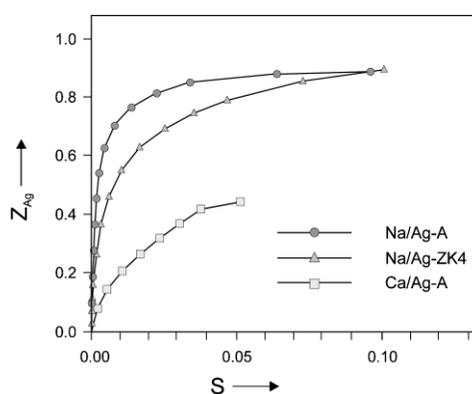
**Fig. 5** Ion exchange isotherms for the systems  $\text{Na}^+/\text{Ag}^+$ -A,  $\text{Na}^+/\text{Ag}^+$ -ZK4 and  $\text{Ca}^{2+}/\text{Ag}^+$ -A at room temperature, where  $Z_{\text{Ag}}$  is the exchange degree inside the zeolite and  $S$  is the equivalent fraction of  $\text{Ag}^+$  in solution.<sup>15</sup>
