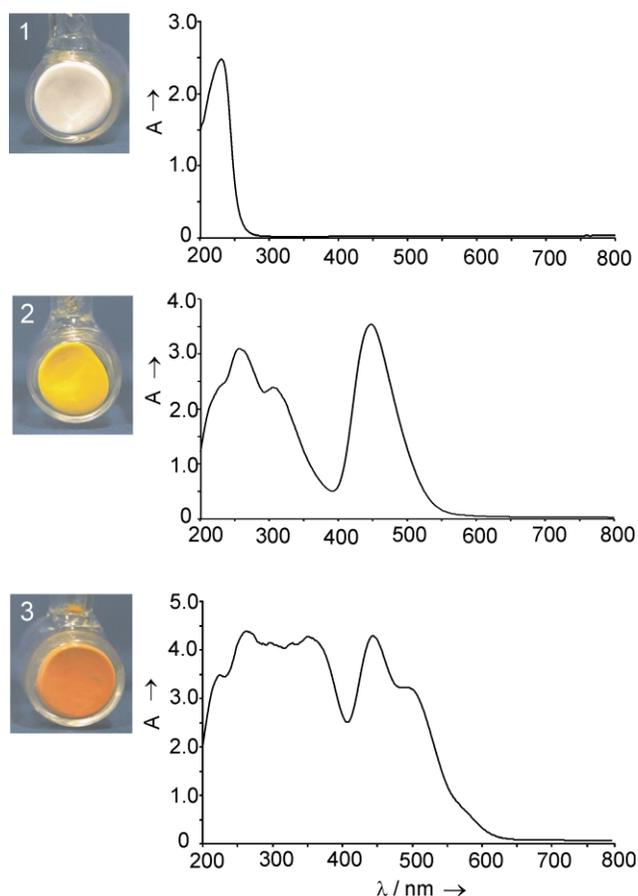
**Fig. 9** Samples (left) and the corresponding UV/Vis spectra (right) of  $\text{Ag}_6^+\text{Na}_6^+\text{A}$  in its fully hydrated state (1), after activation in high vacuum at room temperature (2), and after activation in high vacuum at 200 °C (3).
