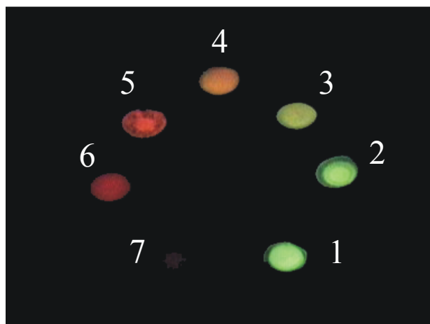
Figure 28. Photographic picture of the fluorescence of dye loaded zeolite L layers upon monochromatic irradiation at 485\pm 5 nm and observation through a 500 nm cutoff filter. 1 and 7 are references loaded with Py^+ and Ox^+ only. 2 to 6 contain a 1:1 mixture of Py^+ and Ox^+ of the following concentrations: 2 , 2.50\cdot 10^{-4} M; 3 , 1.25\cdot 10^{-3} M; 4 , 2.50\cdot 10^{-3} M; 5 , 5.00\cdot 10^{-3} M; 6 , 1.00\cdot 10^{-2} M.
