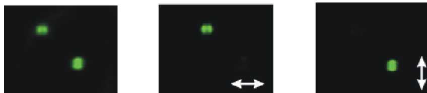
Figure 10. Fluorescence microscopy picture of two 1500 nm long zeolite L crystals containing DSC. Excitation with unpolarized light at 480 nm. Left: unpolarized observation. Middle and Right: linearly polarized observation. The arrows indicate the polarization direction.
