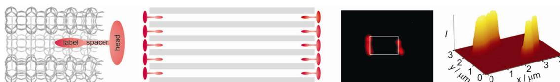
Figure 2. Stopcock principle. Left: A channel entrance with a schematically represented stopcock molecule. Middle: Schematic representation of a zeolite crystal plugged with stopcock molecules at the channel entrances. Right: Confocal fluorescence microscopy images of an ATTO680-zeolite L crystal. The two images indicate that only the base of the crystal is modified with ATTO680. The zeolite crystal is marked with a rectangle in the image on the left side.
